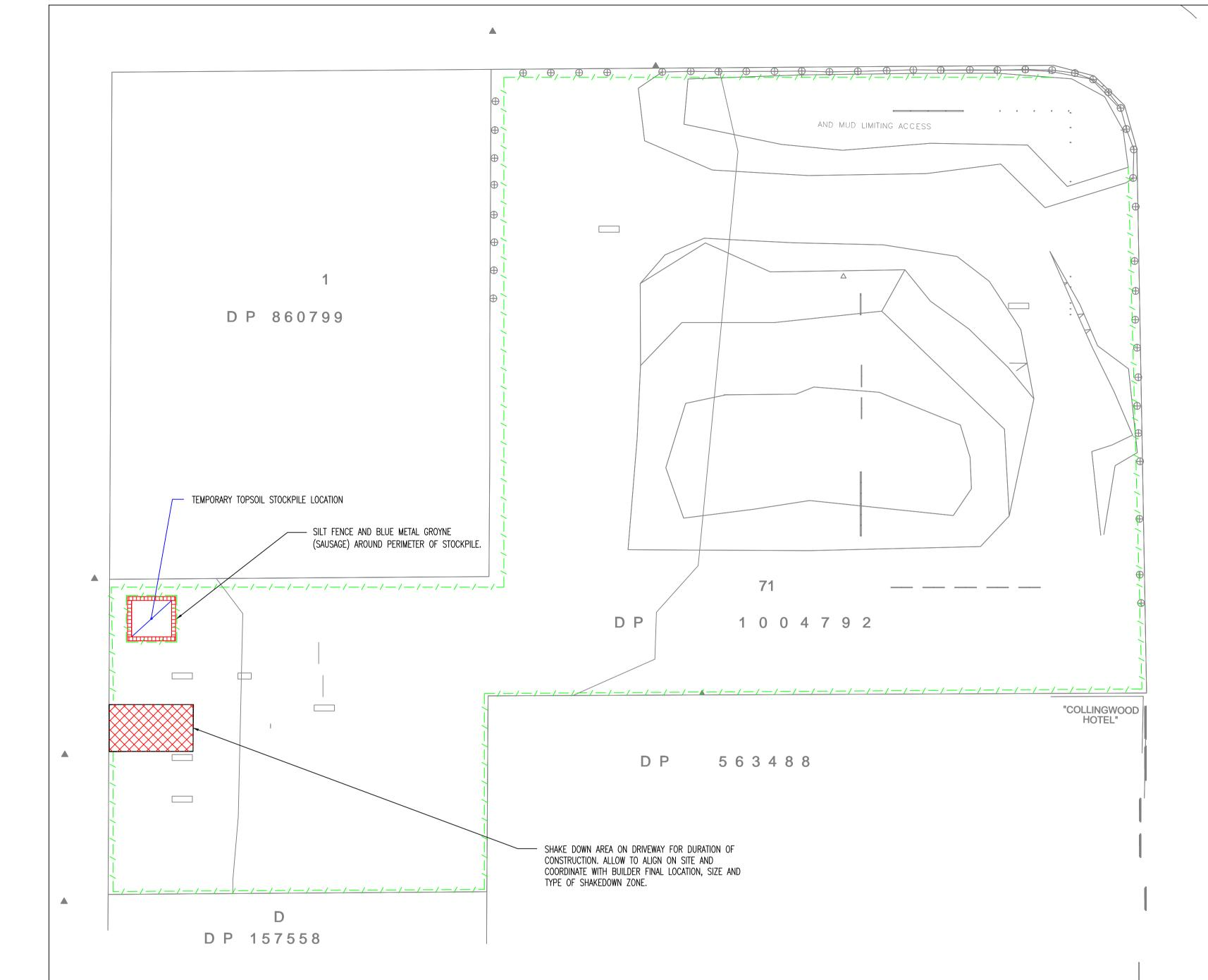
1. EROSION AND SEDIMENT CONTROL DEVICES ARE TO BE MAINTAINED BY THE CONTRACTOR DURING CONSTRUCTION WORKS. 2. ALL RAINWATER MUST BE DIRECTED TO TEMPORARY PUMP OUT PIT. PUMP OUT PIT MUST BE FITTED WITH FILTRATION DEVICE. ALL PUMPED WATER MUST PASS THOUGH FILTRATION DEVICE PRIOR TO BEING PUMPED.
